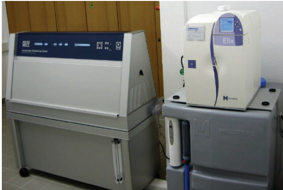
Figure 3: Accelerated weathering tester QUV/SPRAY and water treatment plant type ELIX 15
