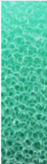
Open cell foam 75x magnified
