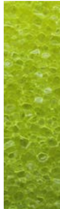
Closed cell foam 75x magnified
